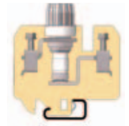
Connection of internal metallic parts
