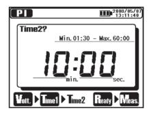
The instrument gets into the Stand-by Mode when settings are made. Setting items for PI measurement are as follows. Refer to the **Setting for Measurement** (=>P.30) and change settings.
